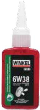
*It is a fast-curing, high-strength compound developed especially for all kinds of cylindrical connections exposed to static shear strength and dynamic loads. When the product is used between metal threads and in an airless environment, it reacts and cures. It has resistance to temperature up to 180°C. It is widely used to bond gear wheels, pulleys and rotor joints.*
