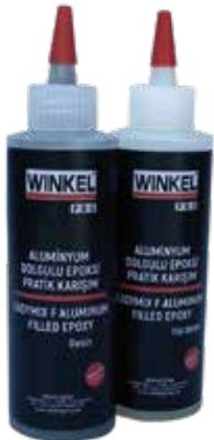
*It is an aluminum filled surface casting repair epoxy. Suitable for hard and permanent repair in castings. It is a grey colored epoxy resin especially developed for casting in gaps between 0,4 and 12,5 mm. When hardened, it can be drilled or machined using conventional metalworking tools.*
